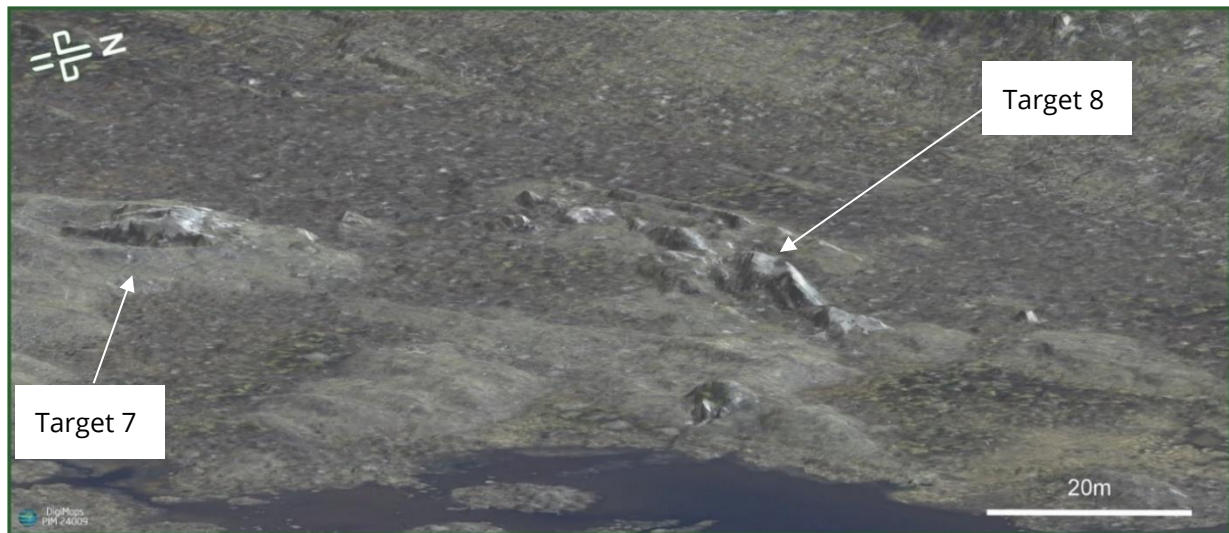
Figure 3: 3D render of digital terrain model (DTM) draped with LIDAR of priority targets (true elevation) – Note That this image was released subsequent to the quarter on 29 July 2024
