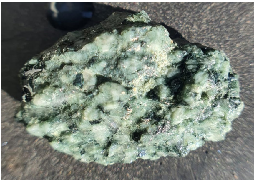
Figure 3: Rock chip from DPRC006 50-51m) highlighting chloritic alteration.
