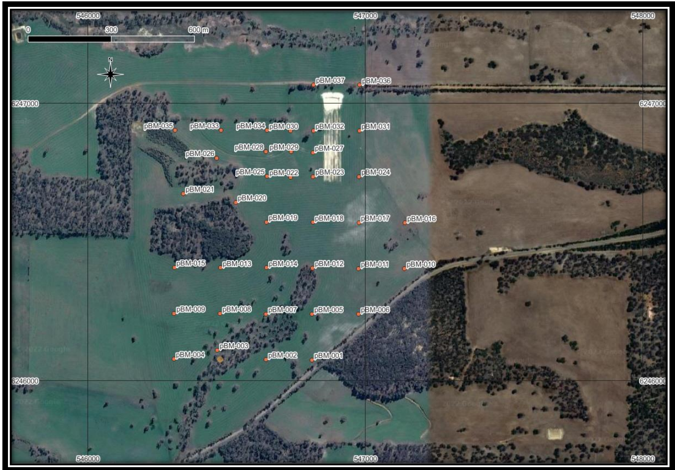
Figure 1: Drill hole location plan at the Bill's Middle target at the Bobalong Kaolin Project
