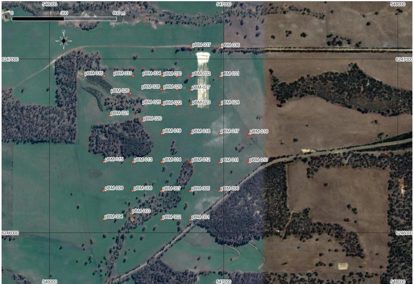
Figure 2: Drill hole location plan of first phase of drilling at the Bill's Middle target at the Bobalong Kaolin Project
